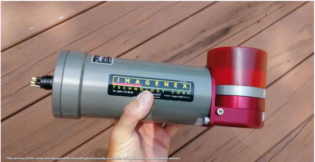
This version of the sonar was designed for mounting horizontally on smaller ROVs. (Courtesy of Paul Unterweiser)
