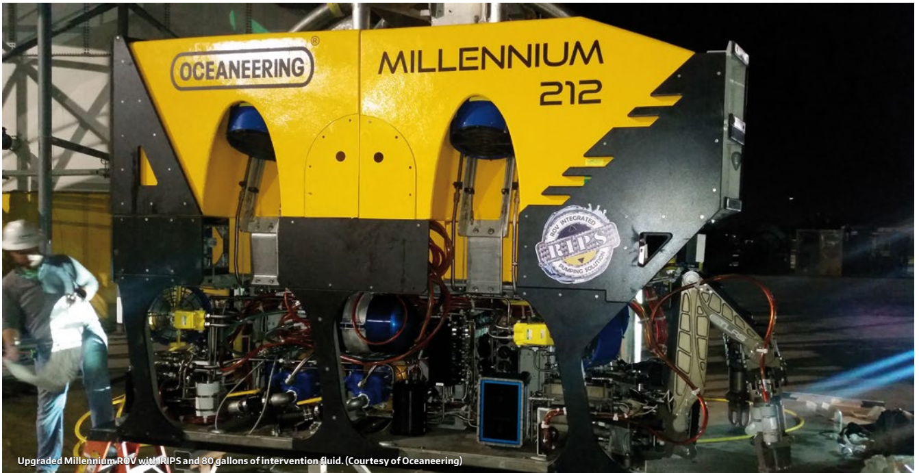
Upgraded Millennium ROV with RIPS and 80 gallons of intervention fluid. (Courtesy of Oceanering)
