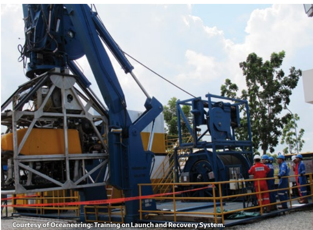
Courtesy of Oceaneering: Training on Launch and Recovery System.
