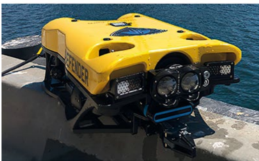
Smart sub-sea inspection with Numurus' NEPI operating system and SeeByte's AI target detection models onboard VideoRay's Mission Specialist Defender ROV. Photo credit: Numurus and VideoRay
