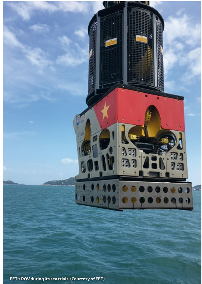
FET's ROV during its sea trials. (Courtesy of FET)
