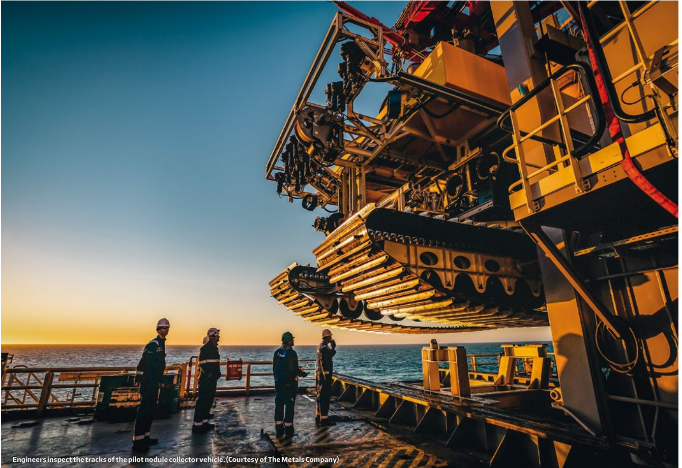
Engineers inspect the tracks of the pilot nodule collector vehicle. (Courtesy of The Metals Company)
