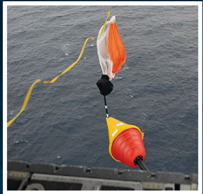
LBI Air-expendable Ice Buoy (AXIB) and parachute being deployed over Beaufort Sea via C-130 platform. (Courtesy of USNIC)
