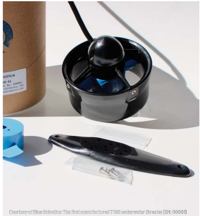
Courtesy of Blue Robotics | The first manufactured T100 underwater thruster (SN: 00001)
