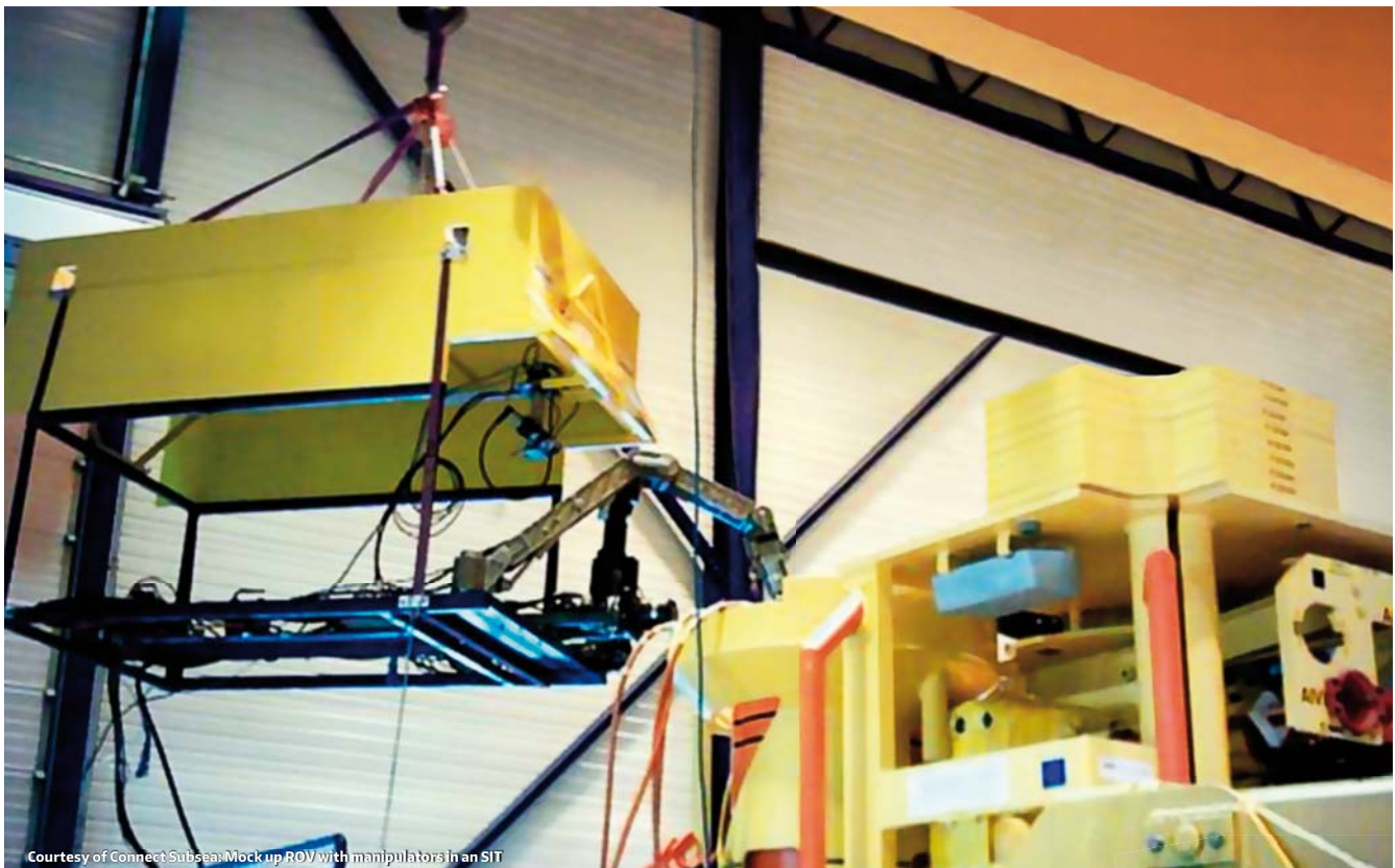
Courtesy of Connect Subsea: Mock up ROV with manipulators in an SIT
