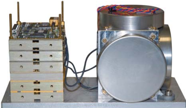
Courtesy of iXBlue: The Internals of an OCTANS
