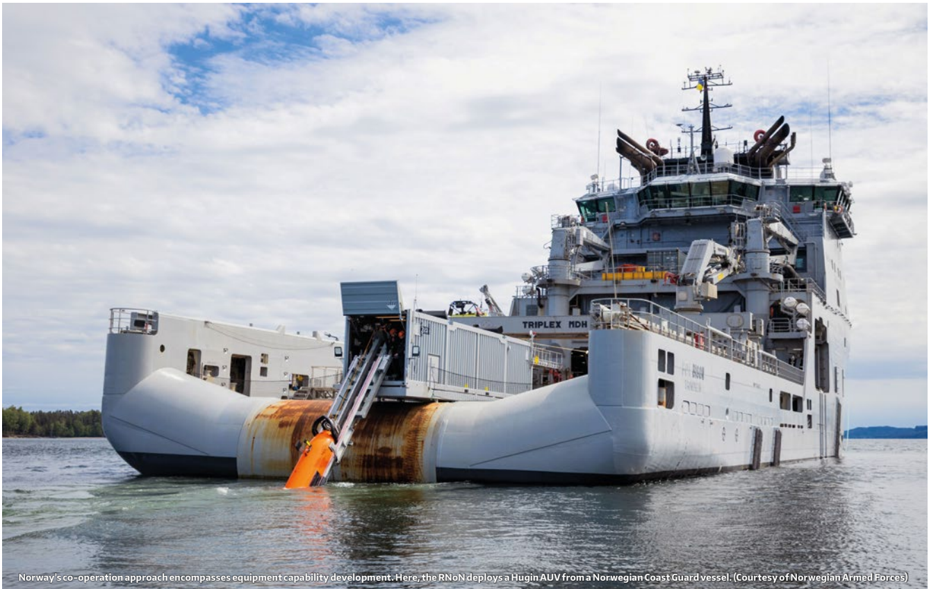
Norway's co-operation approach encompasses equipment capability development. Here, the RNoN deploys a Hugin AUV from a Norwegian Coast Guard vessel. (Courtesy of Norwegian Armed Forces)
