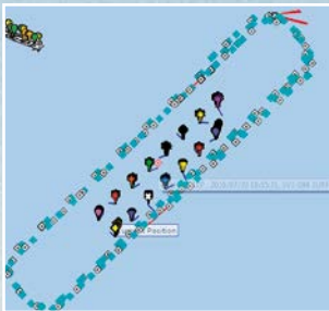
Fig. 4: Graphic display from navigation management system, showing AMVs arranged in a grid pattern around an obstruction (pink square) to collect data while the source vessel (upper corner) follows a racetrack path around the AMV spread, Green Canyon, Gulf of Mexico. (Courtesy of Schlumberger)
