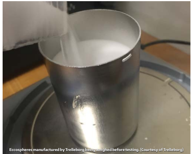
Eccospheres manufactured by Trelleborg being weighed before testing. (Courtesy of Trelleborg)
